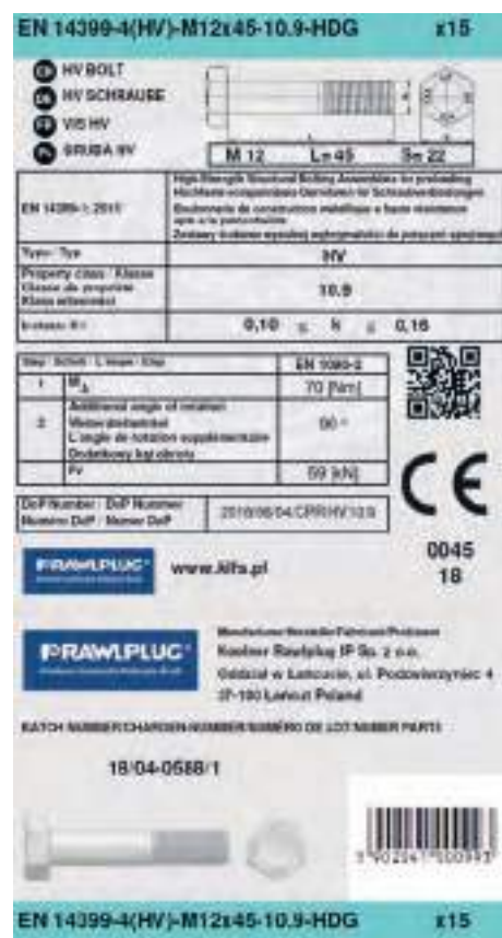
Fig. 11 An example of the label characterizing the bolt for class K1.
